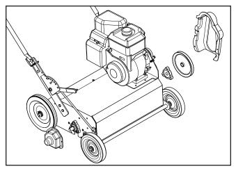
Remove guards and rotor shaft fasteners
